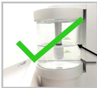
Correct water level, between minimum and maximum lines.
