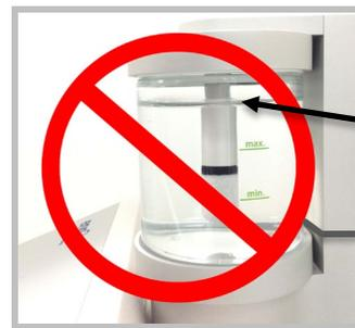
Wrong water level because it is above the maximum line. This would cause water to come out of the FlexArm or Nasal Cannula.
